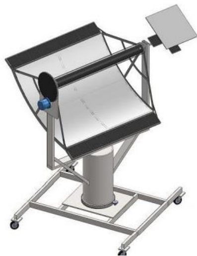
Fig. 4. Structural and mechanical design of the PCST-TSS with dual-axis tracking.
