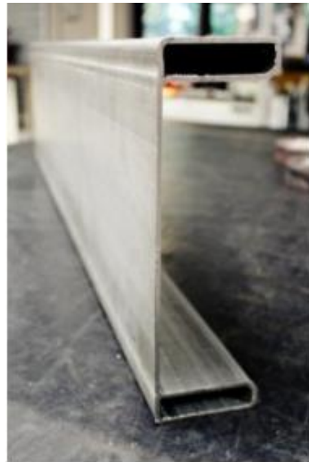
Fig. 1. LiteSteel Beam section profile
