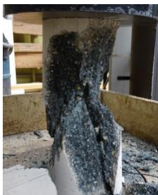
Fig. 17. Concrete cylinder specimen subjected to monotonic compression
