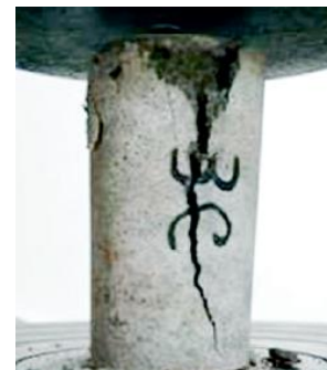
Fig. 3. Column-like mode of failure in plain concrete (Bezerra et al. 2016)
