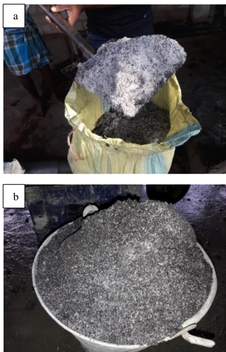
Fig. 1. Types of RHA (a) Long burned (b) short burned
