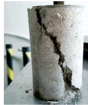
Fig. 2. Shear plane mode of failure in plain concrete (Bezerra et al. 2016)
