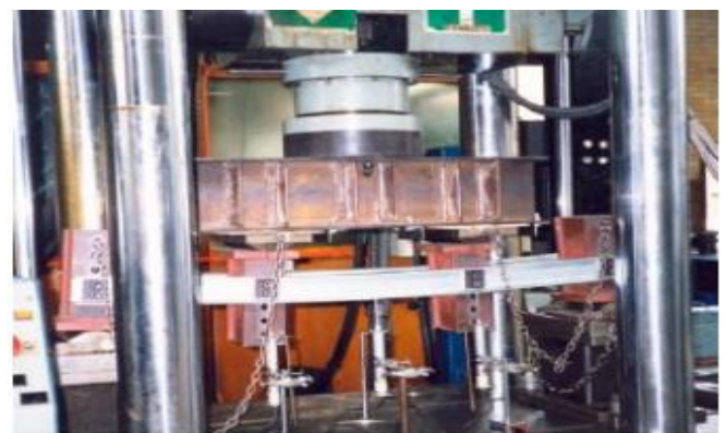
Fig. 4. Bending test set-up [10]
