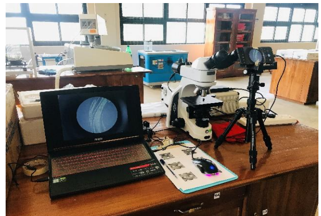
Fig. 1. Morphology investigation setup (Iscope microscope, 10X and 5X magnifying lens kit, 64 Mega Pixel, f/2.0, 29 mm (telephoto lens) mobile camera (Samsung Galaxy S20+).
