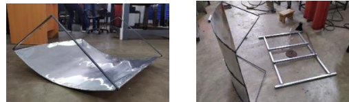
Fig. 8. Reflector (left) and the base (right) of the solar concentrator fabricated at SEUSL mechanical engineering workshop.
