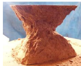
Fig. 4. Hour glass crack pattern of cube (Tripura, D., and Singh, K.D, 2017)
