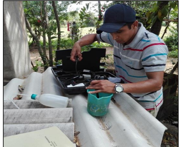
Figure 2 - In-situ measurements of the drinking water samples at the study area
