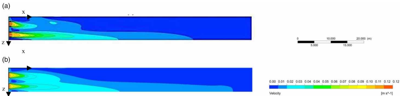
Figure 7 | Velocity contour plot in the xz plane at y = 0.7 m: (a) Stamou & Gkesouli (2015) and (b) computed in this study.
