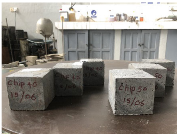
Fig. 7 Compressive strength cubes for chip samples
