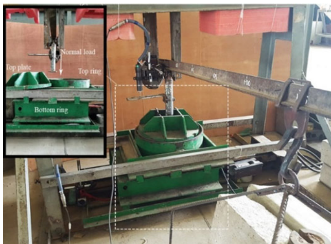
Fig. 2 Large scale direct shear test apparatus
