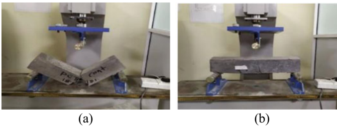
Fig. 8 After the flexural strength test a without PET fibers, b with PET fibers
