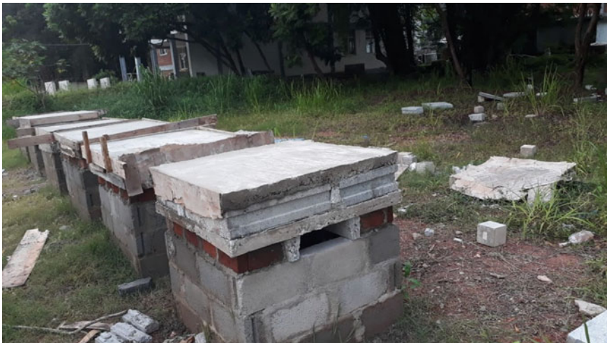
Fig. 1 Proposed insulated NERD slab system
