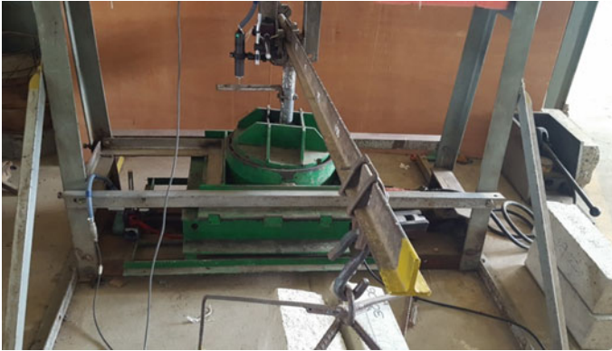
Fig. 2 The large-scale direct shear apparatus
