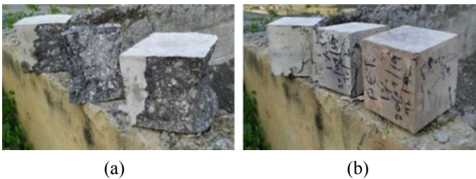
Fig. 4 After the compressive strength test a without PET fibers, b with PET fibers
