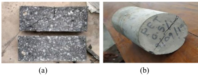
Fig. 6 After the split tensile test a without PET fibers, b with PET fibers
