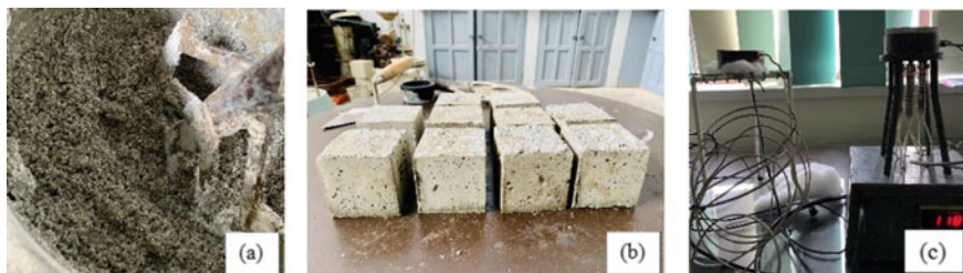
Fig. 3 Specimen preparation and testing a) mixing mortar; b) compressive strength test samples; c) testing thermal conductivity
