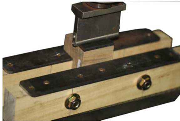
Fig. 2 Shearing tool used for the shear test
