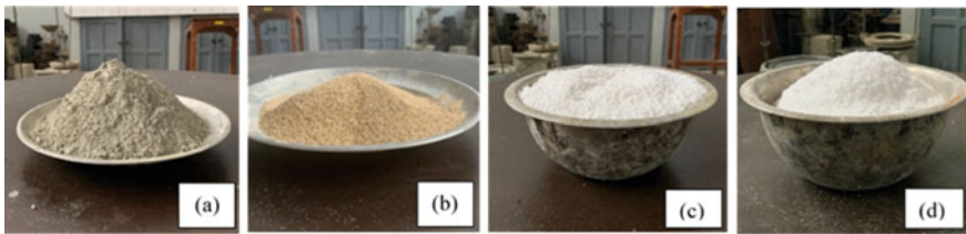
Fig. 2 Materials a) cement; b) river sand; c) EPS—3.35 mm; d) EPS—1.15 mm
